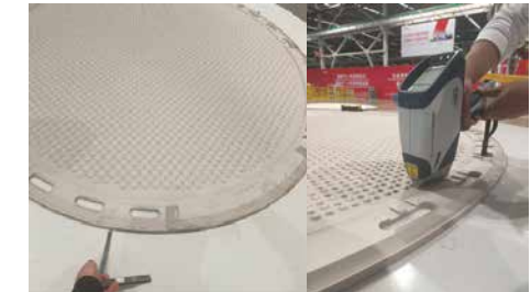
Flatness and Coating Testing
